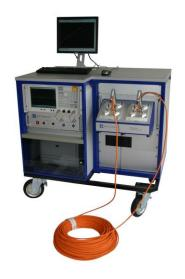
For convenience or operational reasons, it is possible to add a professional movable trolley to the system. In such a case, all tester components are integrated in the trolley, including the computer system and the printer.
